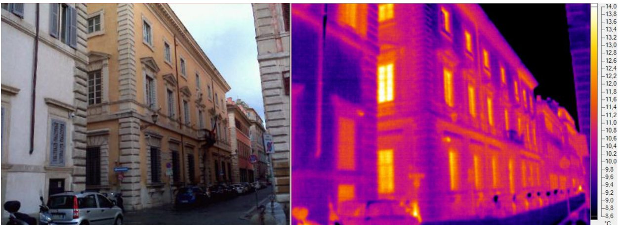
Fig. 7. Comparison between the photography and the termographic image of the main façade of Palazzo Maffei-Borghese, Rome.
