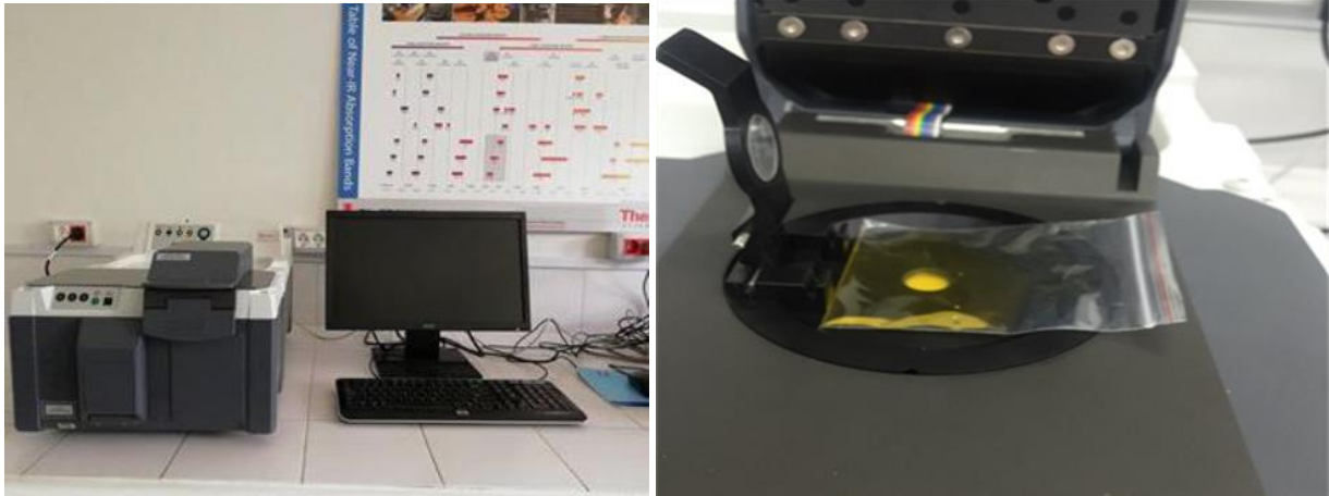
Images 3: The Antaris FT-NIR Analyzer (left) and the sample bag inserted in the machine (right) (by Wadih Skaff)
