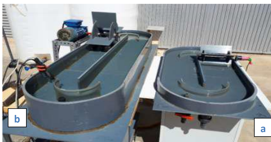
Raceway Pond Reactors of 5 cm (a) and 15 cm (b) liquid depth
