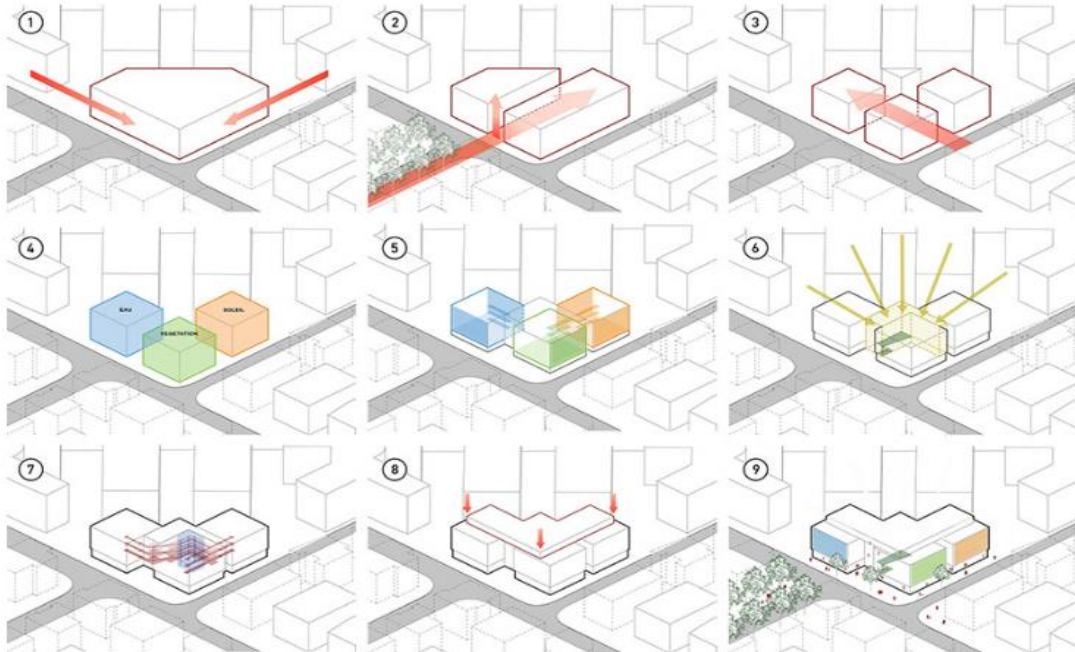
Figure 14: Dividing the building into three cubic parts
