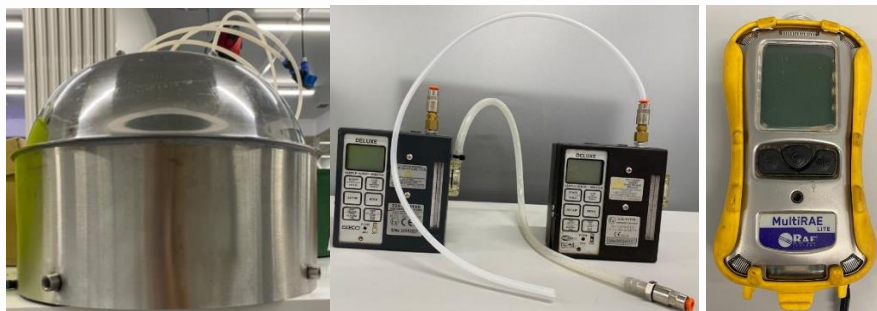
Figure 4 Flow chamber (FC) manufactured by Scentroid (IDES Canada Inc., ON, Canadá- Universal pump- MultiRAE Lite analyser equipment.
