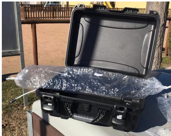
Figura 12 Bag or odour sampling Data Source Provider: DECOST Project (UVIC-Beta Technology Center)
