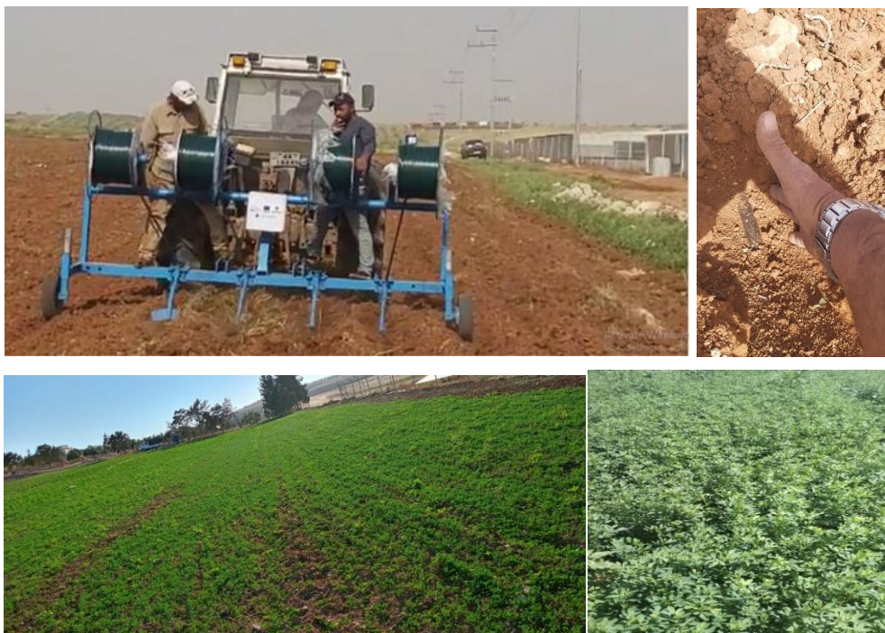
Figure 8. NARC designed and developed a local machine for sub-surface drip irrigation system installation
