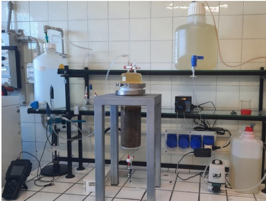
Figure 18. Setting up the flow-through column experiment
