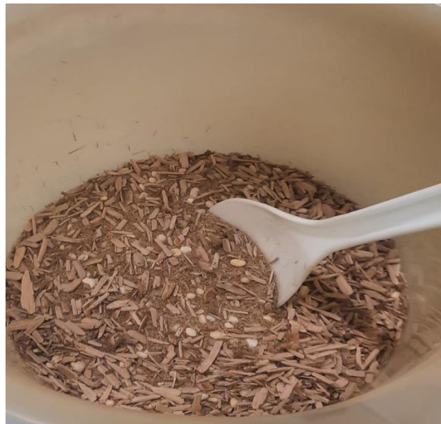
Figure 17. A mixture of sand, gravel, and eucalyptus wood chips
