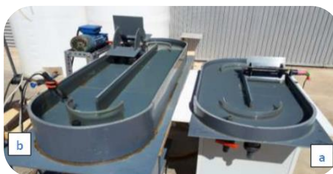
Figure 20: Raceway Pond Reactors of 5 cm (a) and 15 cm (b) liquid depth. Source: Ms Amal Mejri Phd Thesis
