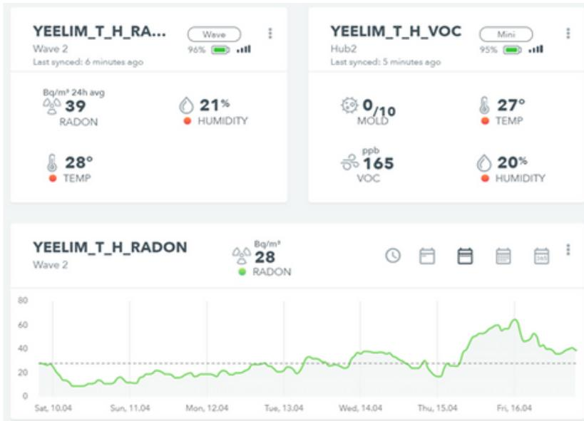
*The installed equipment measures indoor temperature, relative humidity and concentration of radon gas. The results refer to the example of measurements and the graph refers to the weekly history of radon gas measurement.*
